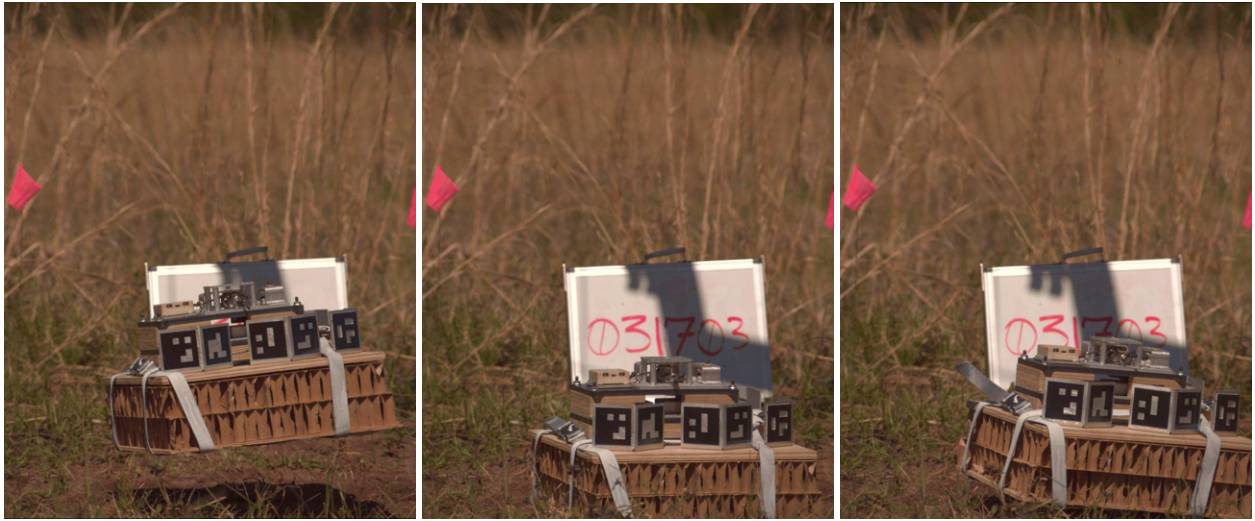
Fig. 13 A cardboard honeycomb impact: (left) before ground contact, (center) at maximum crush depth, (right) at max rebound height
