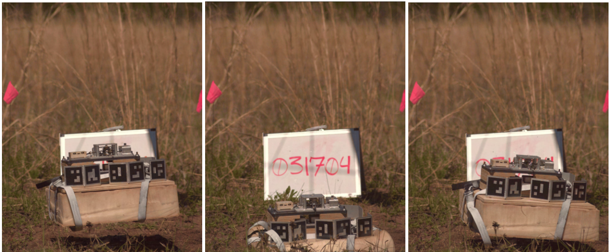
Fig. 14 A soft poly foam impact: (left) before ground contact, (center) at maximum crush depth, (right) at max rebound height
