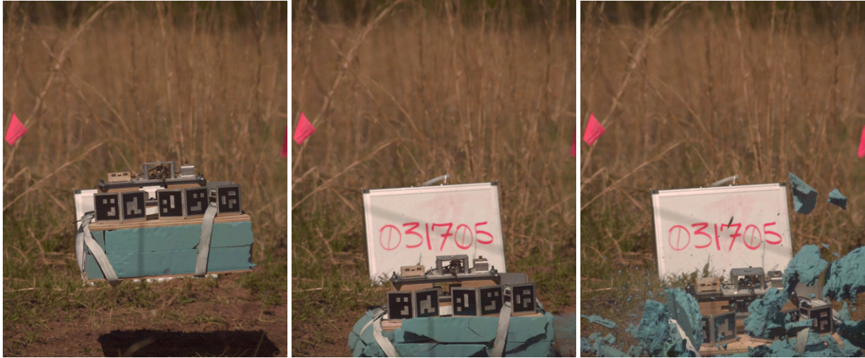
Fig. 15 An impression foam impact: (left) before ground contact, (center) at initial ground contact, (right) at final crush depth
